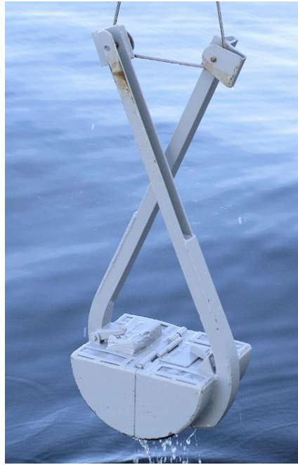
Figure 5.7 A Van Veen grab works like a claw to grab sediment containing macrofauna from the seafloor.
