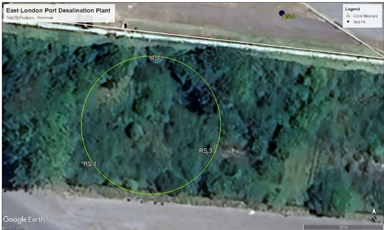
Figure 6: Reservoir– Trial Pit Layout
