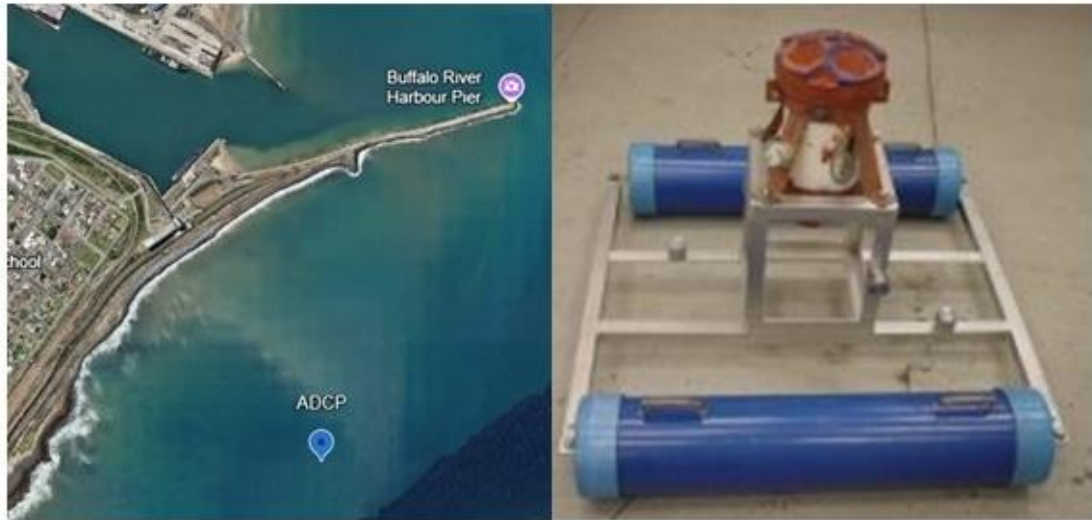
Figure 5.2. Configuration of the SonTek Argonaut ADCP bottom mounted mooring deployed outside of the East London Harbour for an operational period of 37 days.
