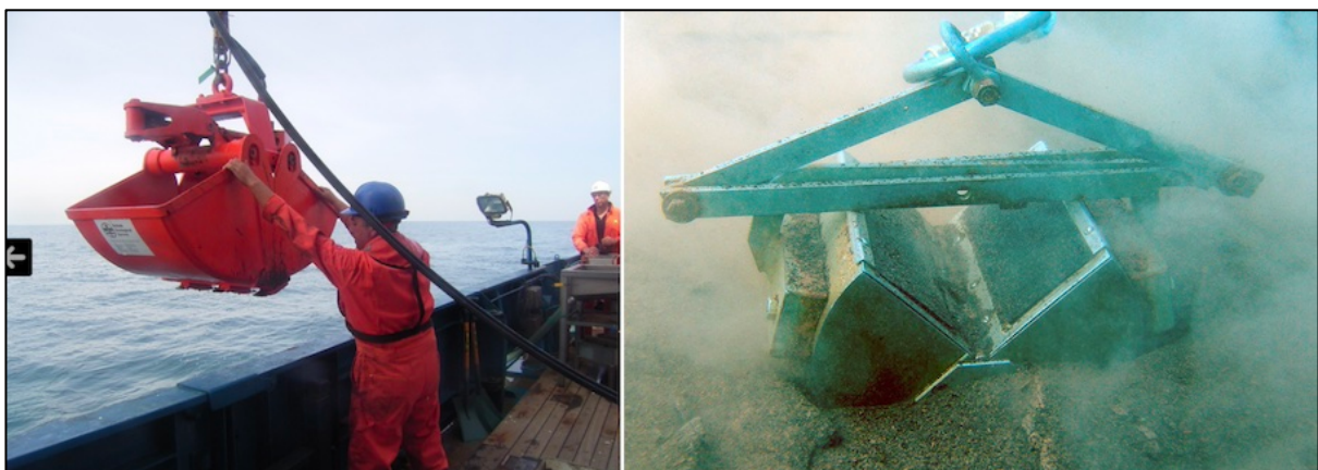
Plate 4: Examples of clamshell grab being deployed (Source: https://ets.wessexarch.co.uk/recs/how-we-study-the-seafloor/geological-methods/# and https://www.researchgate.net/publication/363275000_You%27re_going_to_do_What_Where_Challenges_for_resource_estimation_on_the_Chatham_Rock_Phosphorite_Project/figures?lo=1 ).
