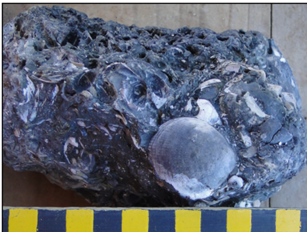
A3-2. Example of cemented Miocene hardground with shell moulds.
