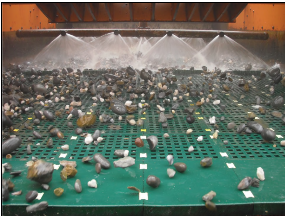
Figure 8. The gravel oversize screen on a typical diamond mining vessel where the geological personnel monitor the material being dredged and where fossil collection takes place.
