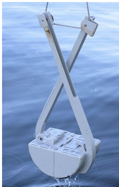
Figure 2.6 A Van Veen grab works like a claw to grab sediment containing macrofauna from the seafloor.
