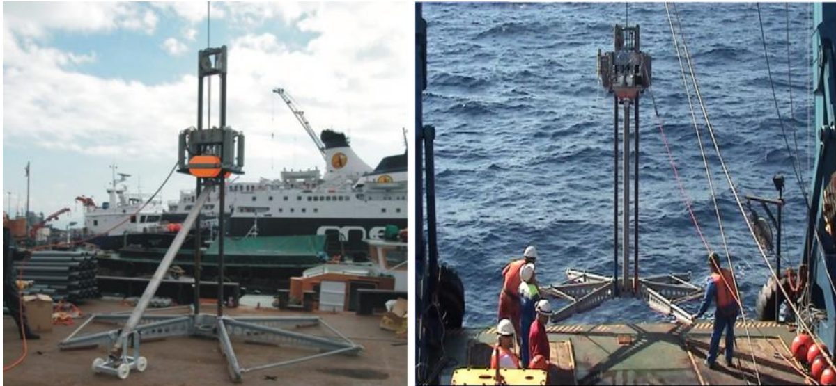
Figure 2.8. Left: An example of vibracorer instrument used to sample sediment samples from the seabed; Right: A vibracorer being deployed from a sampling vessel (image sources: GEO Marine Survey Systems, 2011).
