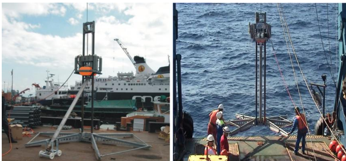
Figure 4.8. Left: An example of vibracorer instrument used to sample sediment samples from the seabed; Right: A vibracorer being deployed from a sampling vessel (image sources: GEO Marine Survey Systems, 2011).
