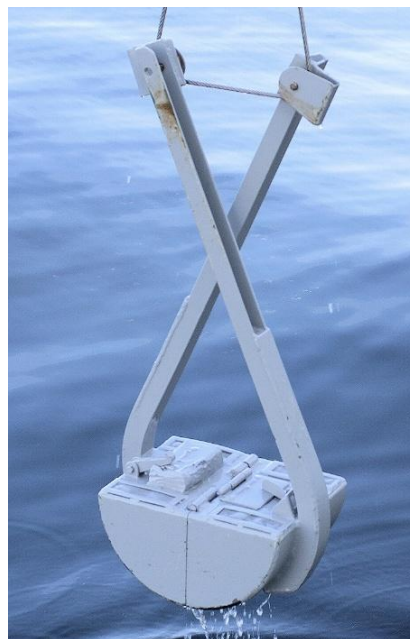
Figure 4.6 A Van Veen grab works like a claw to grab sediment containing macrofauna from the seafloor.
