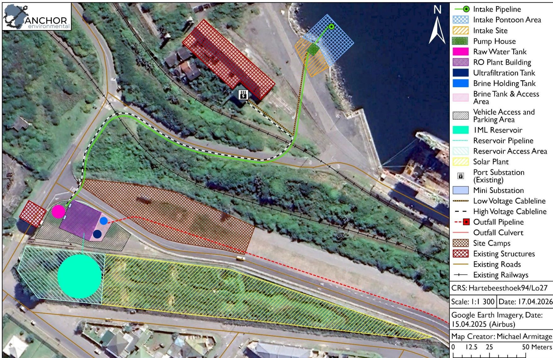
Figure 4.3. The intake, RO Plant, Solar Plant, and all supporting infrastructure.
